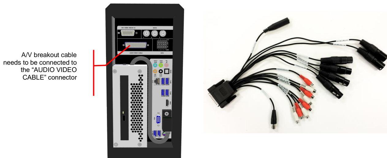
Figure 10 – Cbox P3 | A/V Breakout Cable
