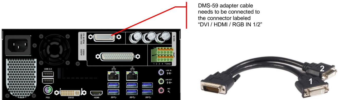
Figure 26 – Cbox S3 Plus (Breakout Cable version) | DMS-59 Adapter Cable
