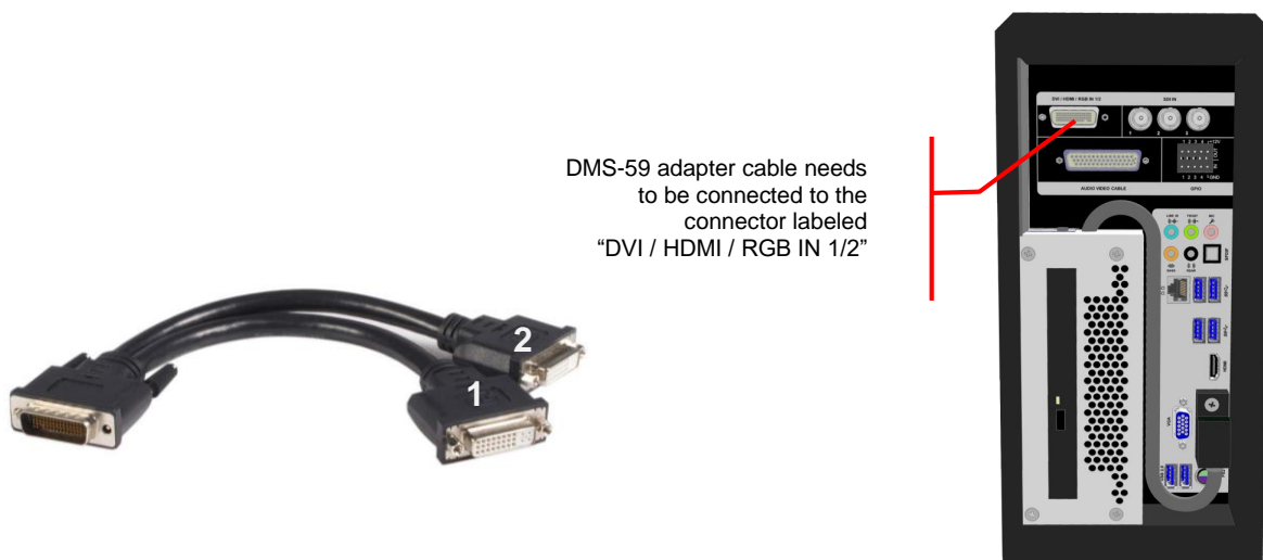
Figure 12 – Cbox P3 | DMS-59 Adapter Cable
