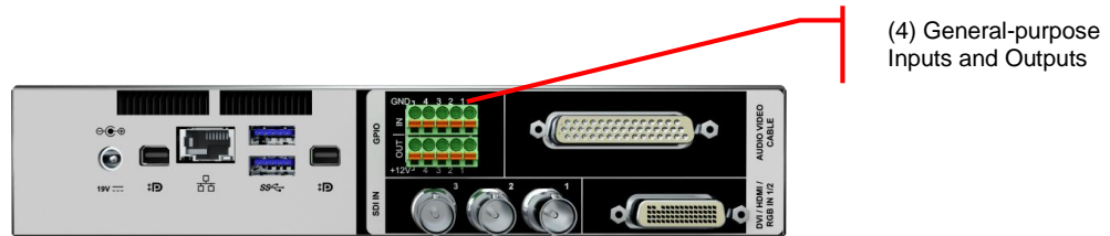
Figure 62 – Cbox L3 | General-purpose Inputs and Outputs
