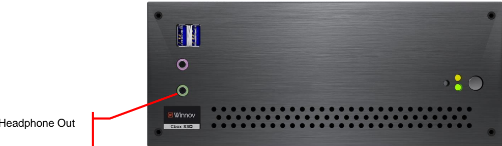
Figure 30 – Cbox S3 Plus | Front Panel / Headphones
