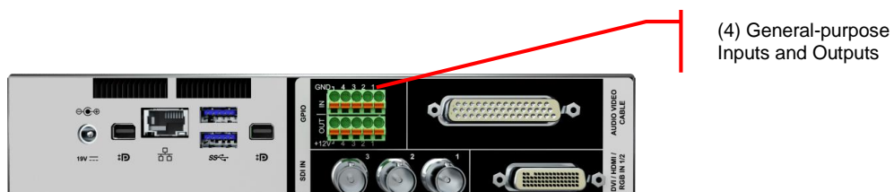
Figure 47 – Cbox S3 | General-purpose Inputs and Outputs
