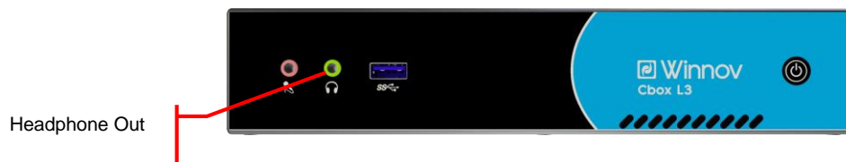
Figure 60 – Cbox L3 | Front Panel / Headphones
